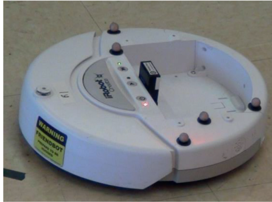
Figure 1. iRobot Create platform.
