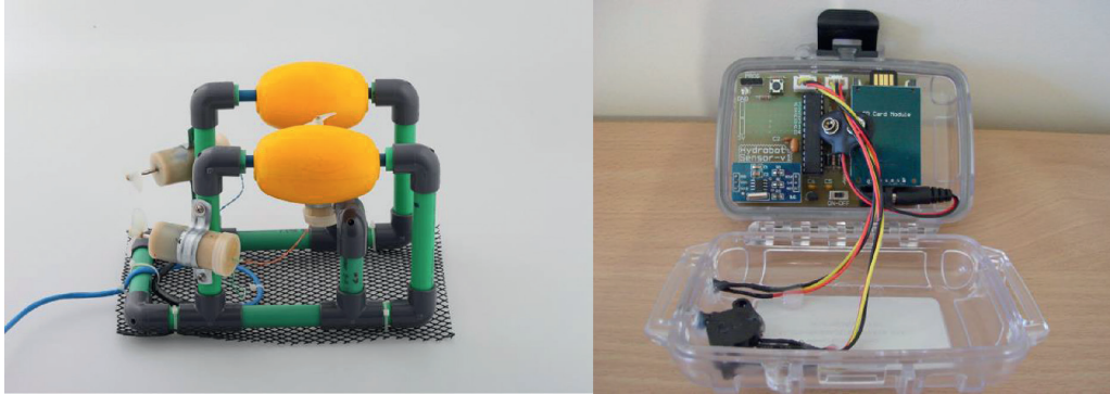
Figure 1. (left) The underwater remotely operated vehicle (ROV), the Hydrobot. Its dimensions are: Length: 28 cm, Width: 16 cm, Height: 19 cm. The construction steps of Hydrobot are described in full details at https://olcms.stem4youth.pl/content_item/detail/12 . (right) The Hydrosensor circuit unit in its waterproof case. Several teams upgrade their ROV by using this sensor kit. The Eugenides Foundation provides this equipment to all the Greek school teams that express their interest. The basic kit consists of the vehicle frame fragments, the motors and the electronic parts for the remote control.
