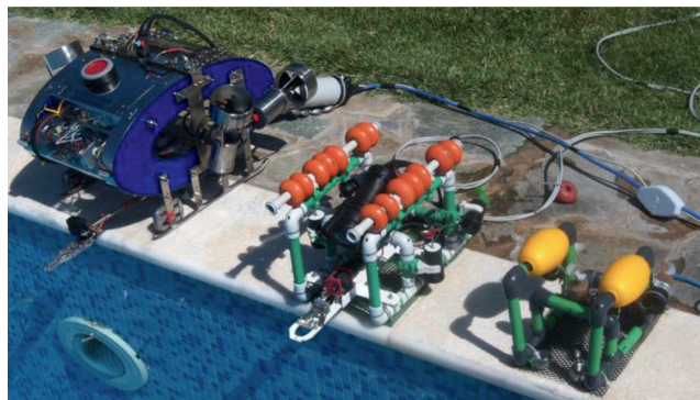
Figure 3. Two of the three upgrades that the team of the 1 st Technical Vocational High School of Salamis island made in Hydrobots. The original vehicle is on the right side of the image. The ROV in the center of the figure has a camera and a gripper. A major upgrade of the initial plan is the vehicle showed on the left side of the figure with four motors and one-degree of freedom gripper. The reader can find more details about the latter at https://www.youtube.com/watch?v=hRsbDD39tik .
