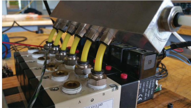
Figure 9. Solenoid valves and orifice block for air engine speed control.
