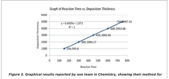
determining the effect of reaction time on film thickness. Note: axis units are missing.
