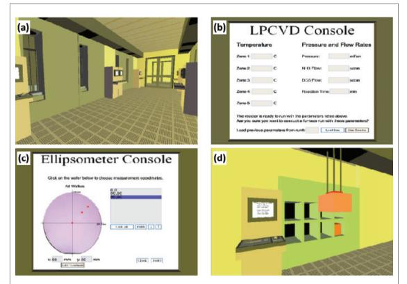
Figure 1. Images of the student interface (a) navigating in the reactor bay, (b) inputting reactor variables to run the reactor, (c) choosing measurement positions in the ellipsometer console, and (d) watching wafers as they load into the ellipsometer.
