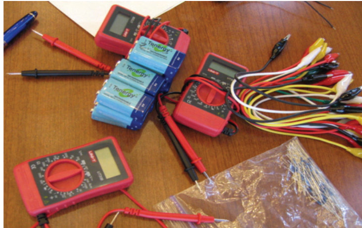
Figure 1. Equipment needed for Module 1, Lesson 4, Potential Dividers. The Lesson demonstrates how potential divider circuits can be used to change the output characteristics of a sensor.
