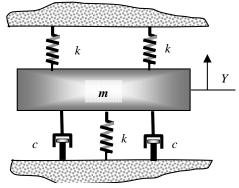
1) Assumptions: Assume no deformation in the springs to make system fit within the supports (no static pre-stressing)
