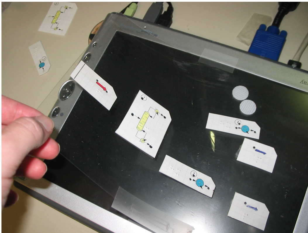
Figure 2. Tablet PC with design medium layer. The computer has a transparency with tactile representations affixed to the material. The Tablet PC has the capability of sensing a left click by tapping and a right click by pushing a button on the barrel of the pen.
